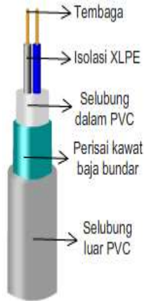
Gambar 2.15 Kabel N2XRGBY
