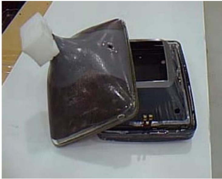
Gambar 5. 9. CRT Components Separated by Saw Cut. Sumber: Kang,H Y et al. 2005
